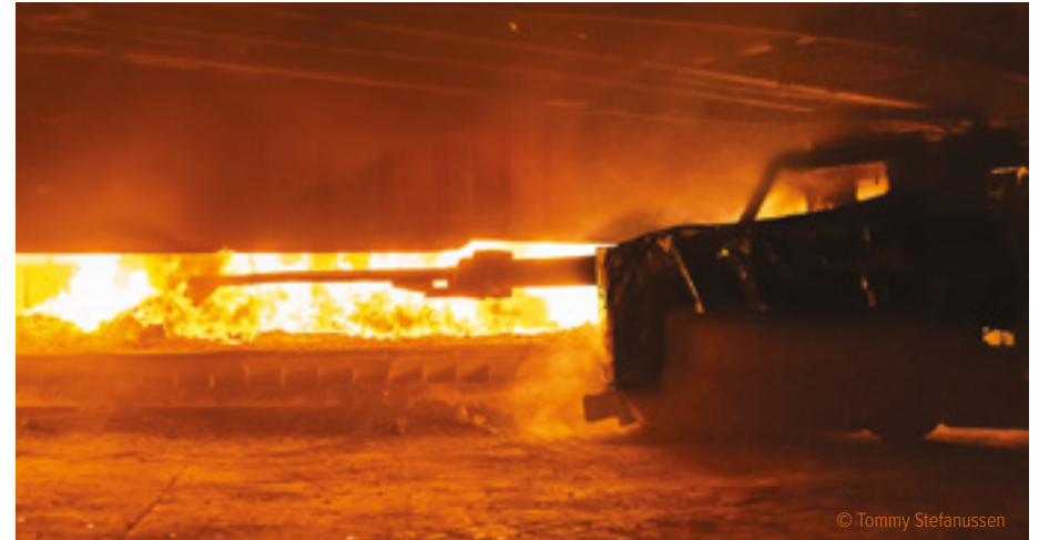
Figure 2: semi-open submerged electric arc furnace
